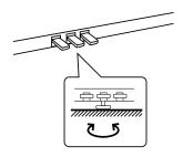
**18.** Turn the adjuster (installed on the bottom of the Pedal Unit) down until it makes firm contact with the floor. If the floor is carpeted, place a spiked furniture cup under the adjuster so that it makes firm contact with the carpet backing. Press any pedal with your foot. If the pedal rail flexes, lower the adjuster until flexing is minimized.
